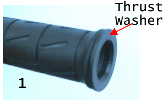
Bar Weight Removed with KAOKO™ Thrust washer in place
