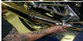
3. Attach TBR slip-tube to TBR muffler using the supplied 6x20mm bolts and lock washers. Leave loose for now.
