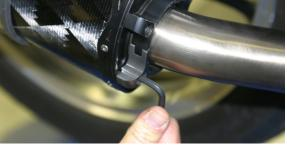
7. Tighten muffler clamp and barrel clamp at slip-tube joint.
