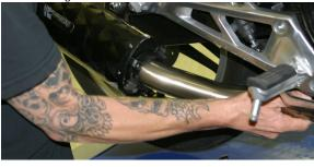
6. Align muffler and tighten the 4 X-ring bolts.
