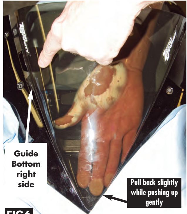
FIG6 Screen Install Front Slot / Right side Wellnut
