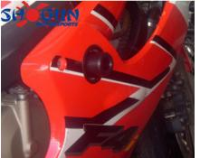
10. Remove right side bolt. Mount right side puck with (99-HB-SH101250110) Socket Cap 10 X 1.25 X 110 Main Engine Stud and torque down.
