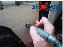
Remove left side bolt. Mount left side puck with (99-HB-SH10125090) Socket Cap 10 X 1.25 X 90 Main Engine Stud and torque down.
